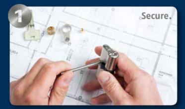
Using the forend screw, turn the MX cylinder at the threaded bore hole through 90° and set the half of the housing, the cam and coupling to the side.
