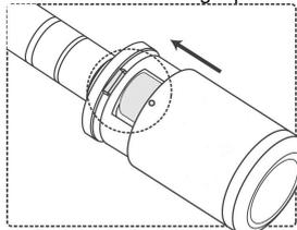
4. Use the mounting tool to hold the nut and turn the cover clockwise on the knob.
