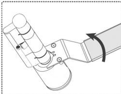
2. Insert the battery into the knob. Please take care that the polarity of the battery (+/-) is like printed in the battery case.
