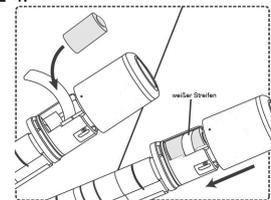
2. Insert the cylinder through the door from outside and fix it with M5 screw to the door **hand-tight**.
