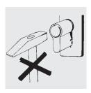
Do not force the cylinder into the lock (with e.g. hammer).
