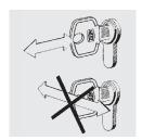
When inserting or removing the key, no lateral forces must be applied.
