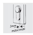
Cylinder should not extend more than 3 mm from the fitting.
